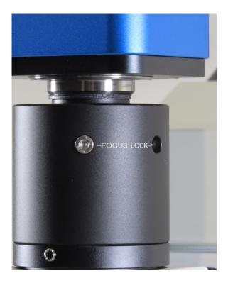
You will note two set screws on the optical coupler itself marked FOCUS and LOCK.
