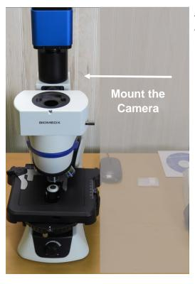
The set screw to hold the camera assembly in place points to the back on the port in this example. On some head assemblies the set screw will be to the side.
