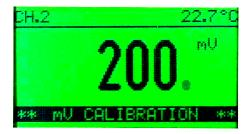
2. Rinse the redox electrode with distilled water, pat dry with a paper towel, and immerse the electrode into a standard solution of known potential - like a 200mV ORP solution. If your electrode is not reading 200mV, adjust the display window to the proper value by simply pressing the up or down arrow to the correct mV potential (200mV) and press CAL.
