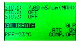
**Note:** If STD.1: which is standard #1, does not have 7.00mS in place, you will need to manually put it there if you are using 7.00mS calibration standard. STD.2 and STD.3 should be turned off. It might take some playing around with the unit to get used to how it works.
