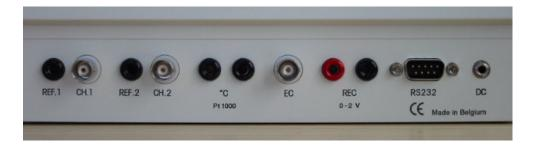
Plug the pH probe into CH. 1, the ORP probe into CH. 2, and the conductivity probe into EC.
