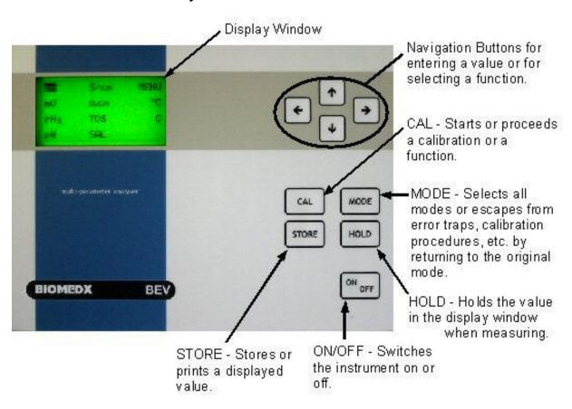
Your first concern when installing a new unit is to plug the probes into the back of the unit, turn it on, go through the initial set-up procedure for your particular preferences, and then calibrate your probes.
