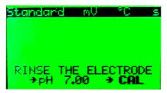
Note that after pressing **CAL** the display is telling you what to do: Rinse the Electrode, put it in a pH 7.00 buffer, press **CAL**. So that is what we do.
