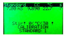
The display instructions will say "Stir!" but we have a small sample size and special probe so this will not be done. The display will blink while calibration is being performed. Once the unit locks into a calibration for the probe, it will shift to the EC mode and present the EC reading. If you had selected another calibration point it would ask for that next calibration solution.
